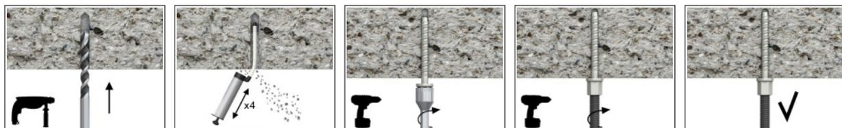
1. Drill the hole with rotary hammer drilling machine. Drill to a required depth.
